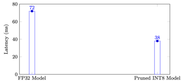
Fig 7. Inference latency before and after model compression.
