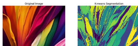
Fig.3. K-Means clustering applied for color segments division of original fabric image into color clusters.
